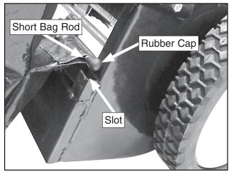
Figure 6. Securing short bag rod.
